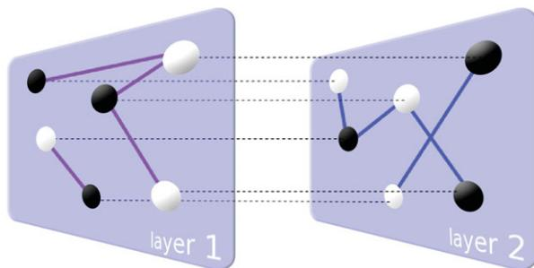
**Figure 1.** Schematic of a two-layer multiplex network. The multiplex is composed of six nodes so that each node appears in each layer and it is connected (dashed lines) with its representation in the other layer. When layers compete, each user must choose the layer in which it is active (black), thus remaining inactive (white) in the other one. (Online version in colour.)
