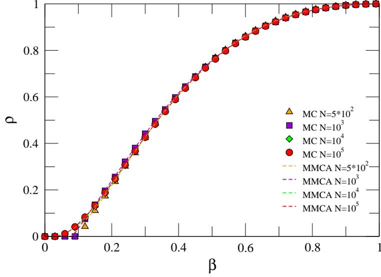
**Fig. 4** Phase diagram for the SIS model ( $\lambda = \infty$ ) in a random scale free network for different system sizes as indicated. The networks have a power-law degree distribution with an exponent  $\gamma = 2.7$  and  $\mu = 1$ . MC results are averages over  $10^2$  realizations. After [26].
