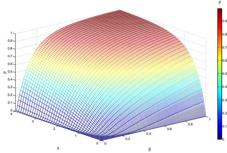
**Fig. 8** Density of infected nodes,  $\rho$ , as a function of traffic flow (determined by  $\Lambda$ ) and the epidemic spreading rate  $\beta$  for BA scale-free networks and a shortest paths routing scheme for packets delivery. Each point is the result of  $10^2$  averages over different networks and initial conditions. After [37].
