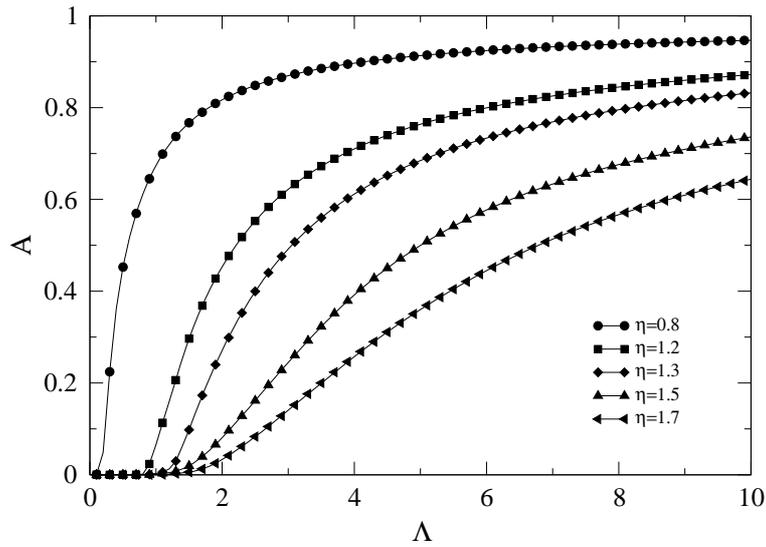
**Fig. 11** Fraction of active packets as a function of the traffic flow with bounded delivery rate. It represents the fraction of active packets  $A$ : packets still traveling in the network over the total amount of generated packets in a time period  $\tau$ , as function of the traffic injected in the system  $\Lambda$  for different values of the delivery capacity  $\eta$ . The underlying network and the routing protocol are the same as in Fig. 7. After [37].
