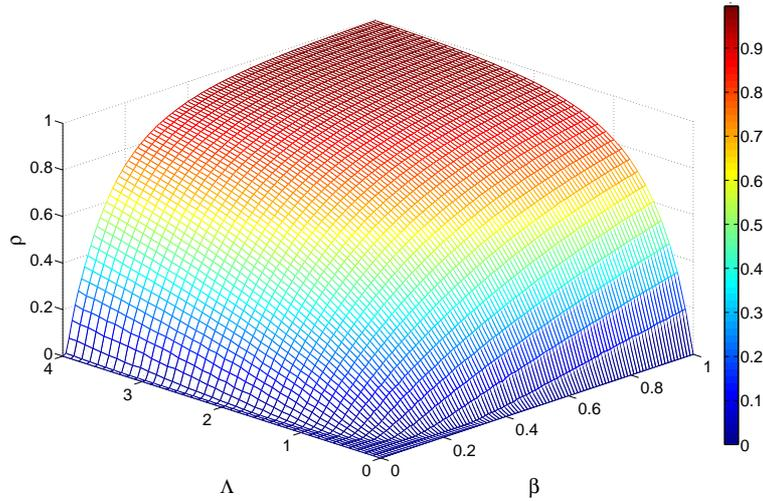
**Fig. 7** Density of infected nodes,  $\rho$ , as a function of traffic flow (determined by  $\Lambda$ ) and the epidemic spreading rate  $\beta$  for random scale-free networks and a shortest paths routing scheme for packets delivery. Each point is the result of  $10^2$  averages over different networks and initial conditions. The exponent of the degree distribution of the network is  $\gamma = 2.7$ . After [37].
