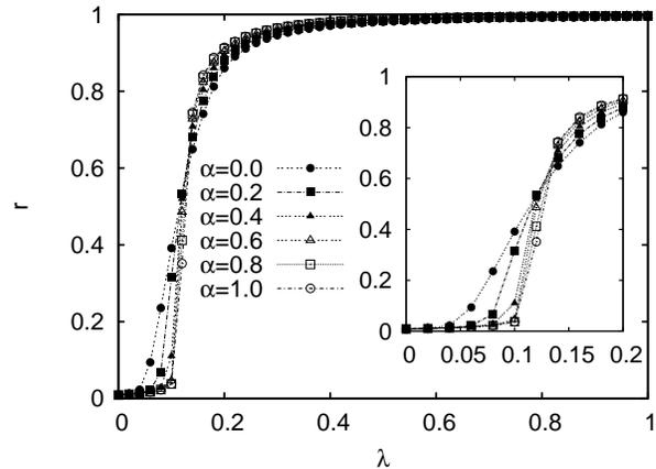
FIG. 1: Global synchronization curves  $r(\lambda)$  for different network topologies labeled by  $\alpha$  ( $\alpha = 0$  corresponds to the BA limit and  $\alpha = 1$  to ER graphs). The inset shows the region where the onset of synchronization takes place. The network sizes are  $N = 10^4$  and  $\langle k \rangle = 6$  ( $N_l = 3 \cdot 10^4$ ) and were generated using the model introduced in [45]
