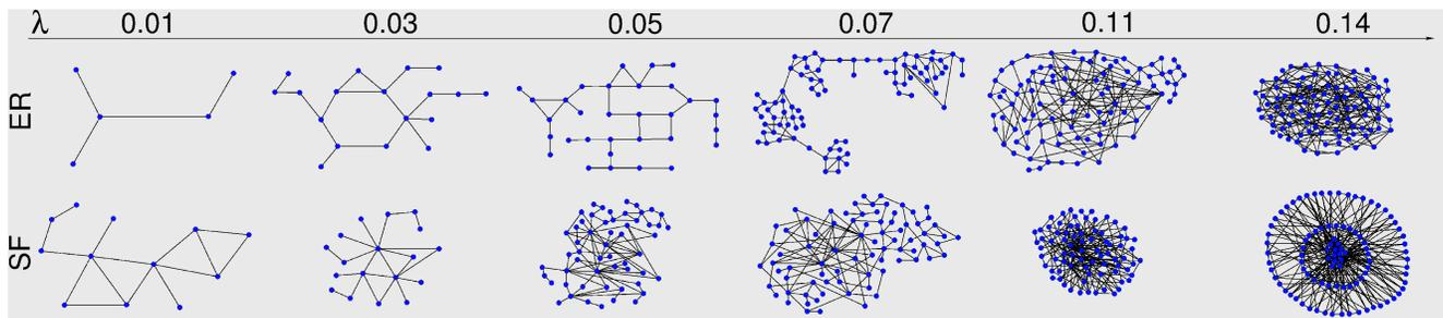
FIG. 4: Giant synchronized components for several values of  $\lambda$  in the two limiting cases of the different topologies studied (ER and SF). The size of the underlying networks is small ( $N = 100$  nodes), in order to have a sizeable picture of the system. Note that for the SF case links and nodes are incorporated together to the  $GC$ , while for the ER network, what is added are links between nodes already belonging to the  $GC$ .
